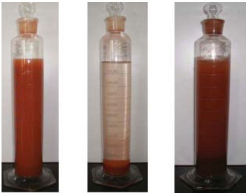
Fig. 4. A typical snapshot showing (a) dispersed phase (b) flocculation/settling of suspended particles in 1 % DP of slime slurry in the presence of natural hard water and (c) stable dispersed phase of 25 % iron ore fines using water from (b) and 0.05 % humate.
